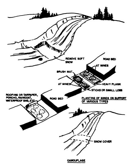
Figure 6-32. Laying mines in deep snow.
