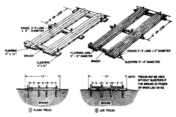
Figure 5-10. Road reinforced with tread.
