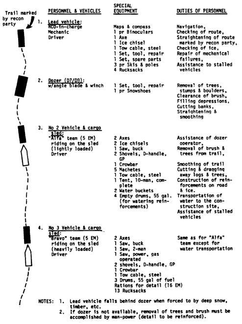
Figure 5-6. Construction detail for winter roads.
