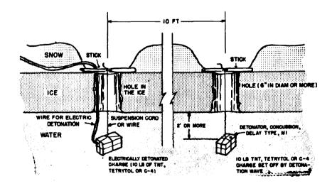
Figure 6-34. Method of placing charges in ice.
