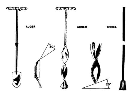
Figure 6-35. Types of ice augers and ice chisel.
