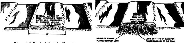
Figure 5-7. Road reinforced with snow.
